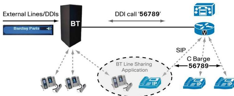
The BT Line Sharing Application is hosted on a Linux appliance server and connects to the Cisco UCM as a SIP phone. SIP is used only for passing the line status between the Cisco UCM and ITS. Audio is passed across a regular DDI call, made over the main SIP trunk connection between the BT system and the Cisco UCM.
